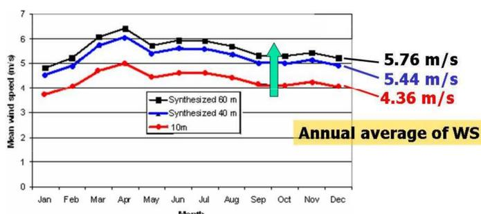
Figure 3. : Mean wind speed variation with altitude
