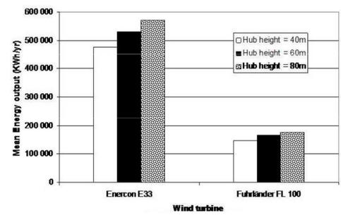
Figure 6. : Mean energy Output for E33 and Fuhrländer FL 100
